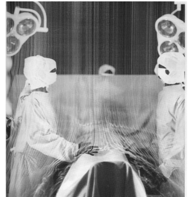
Fig. 6: Laminar displacement flow under a ceiling of an Operation Room.
